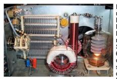
In his days operating under a Part 5 Experimental license, Eric Tichansky, NO3M, ran a modified a Heathkit SB-1000 linear for 630 meters, so he could generate sufficient power to obtain the 100 W ERP permitted under
